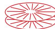
At 180 degrees of rotation, the orifice is completely closed. Adjustable material control from full feed to trickle.
